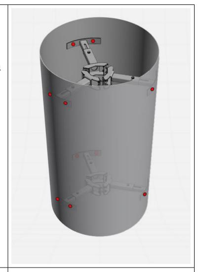
The radome lid is placed on top of the fixed radome and secured with self-tapping screws.
