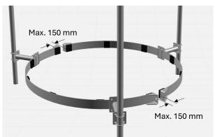
The supplied special U-bolts for hoops must be used to mount the offsets on the hoops.
