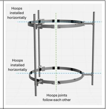
The distance between the flanges in the ends of the barrel band must not exceed 150mm
