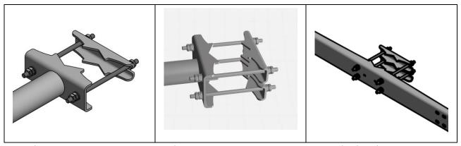
Two-piece collars are assembled with threaded rods. The assembly principle is the same for all types, regardless of whether there are one or two rear parts.
