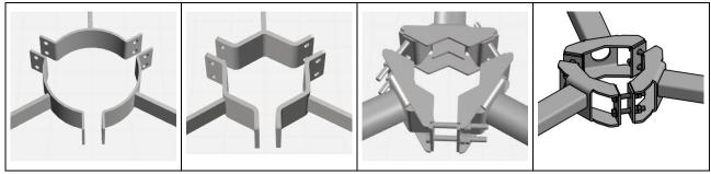
Three-piece collars come in several designs, but the assembly and installation principle is the same for all types.
